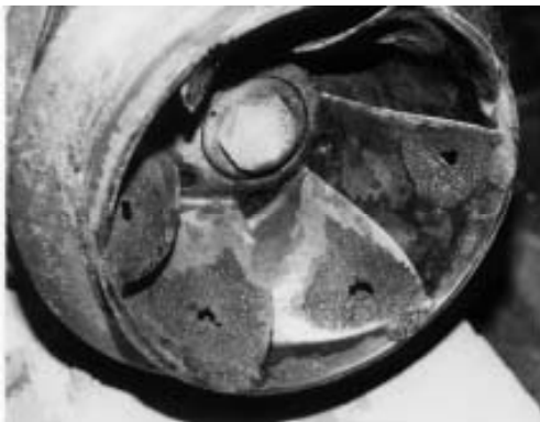
Fig. 1. Erosion of the blades of the mixed-flow pump impeller of Sigma Lutín, the largest Czech manufacturer of water pumps.
